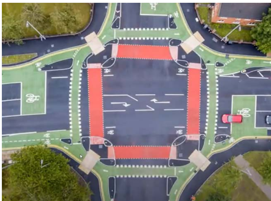
Figure 4 CYCLOPS junction typical layout
